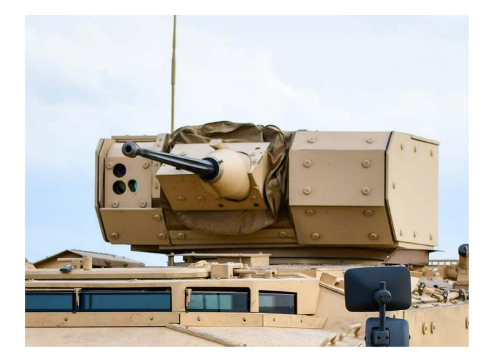
The turret is equipped with an electrooptic sight in order to have effective target
